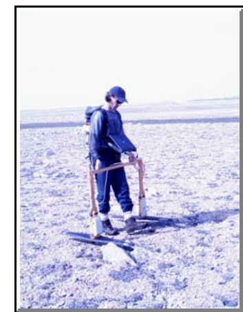
Figure 1. 100 MHz GPR - kimberlite dyke exploration on Victoria Island
